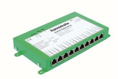
There are 10 sockets/ports on the ZG with 6 I/O lines, 0V and 5Vdc power supply. Each I/O line can be confugured as a digital input or digital output, and some have special function e.g. analog input, analogue output. When configured as digital input lines they have optional 30kOhm pull-up resistors to the 5V supply. Each I/O line has a 130 Ohm inline current limiting resistor and transil over-voltage protection.
