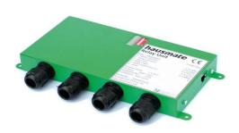
Each relay has a manual over-ride 'ON' switch and an LED indicator to show it is ON. There is also a power supply LED indicator to show the RU is connected to a ZG and has power. The relays are designed to have minimal power consumption, and thus heat generation, by using a larger 'pull-in' current and then reducing to a smaller 'hold' current.
